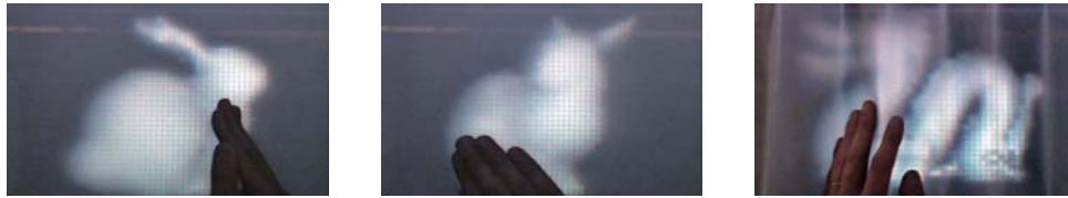
Figure 1: The 3D object that is projected onto the retro-reflective screen can be seen from a number of viewpoints with motion parallax, and the user can operate this object using his/her hands.
